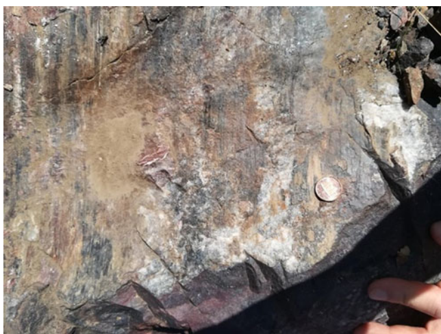
Fig. 2. Typical samples of millimetric orange aggregates, associated with quartz, along a fault plane. They are probably As–Mn minerals characteristic in Valletta Mine.
