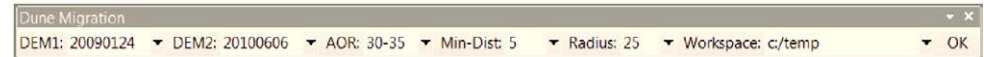
Figure 2. Dune Migration toolbar for the ArcGIS add-in. DEM1—first DEM raster; DEM2—second DEM raster; AOR—angle of repose.
