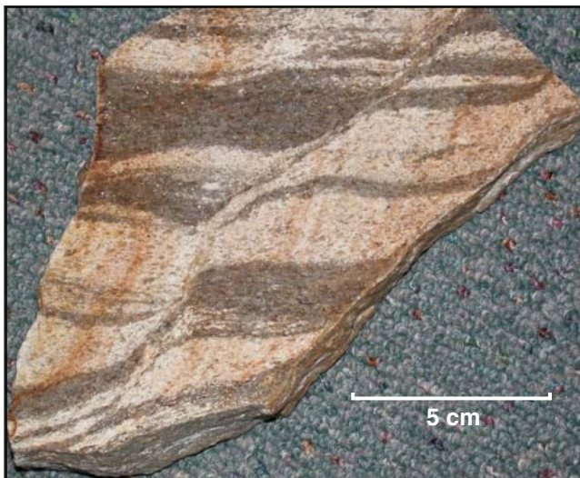
Figure 12. Quartzite hand specimen containing a shear band from the northern Thor-Odin culmination. Note that the overall displacement is not great, but it is sufficient to deflect the surrounding foliation into flanking fault-drag folds. Analogous with the seismic section, some layers are truncated while others curve gradually into the shear band.
