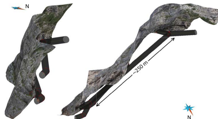
Figure 7. Two perspective views of the tunnels in the subsurface of the north side of the Vajont Gorge. The digital outcrop model is sliced and rotated in order to see the tunnels in the subsurface.
