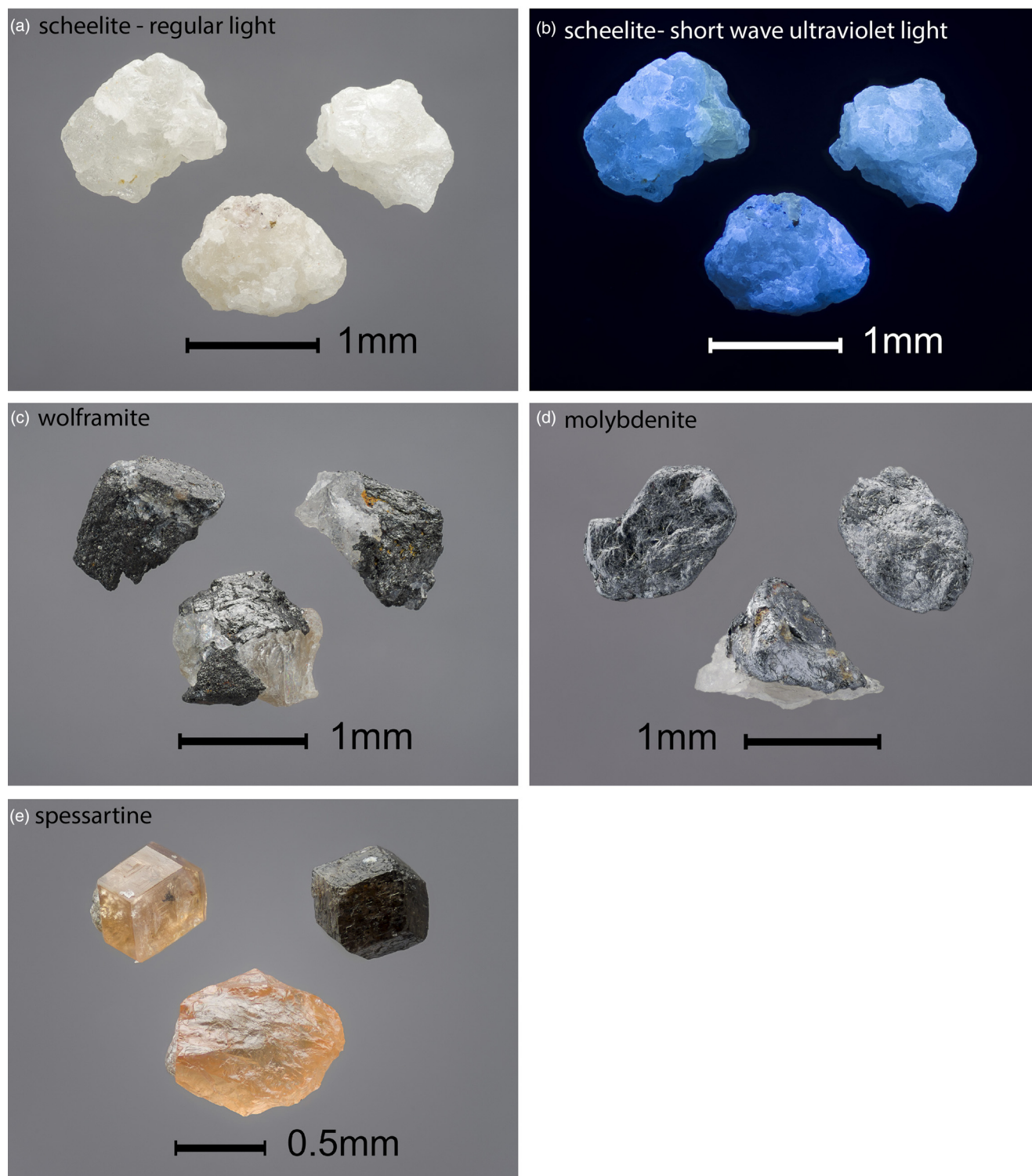
Fig. 4. Colour photographs of indicator mineral grains from till samples from around the Sisson W–Mo deposit: (a) scheelite under visible light from till sample 11-MPB-507; (b) scheelite under short-wave ultraviolet light from till sample 11-MPB-507; (c) black wolframite from till sample 12-MPB-1026; (d) molybdenite from till sample 11-MPB-567; (e) spessartine from till sample 11-MPB-518. Photographs taken by Michael Bainbridge Photography. Please see online version for colour.
